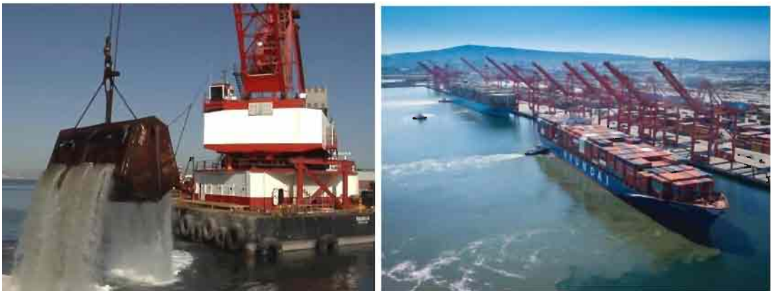
Figure 54. Right, a dredger removing soil and rock deposits around Long Beach Harbour, California USA. LEFT, ships on the Port of Long Beach.
