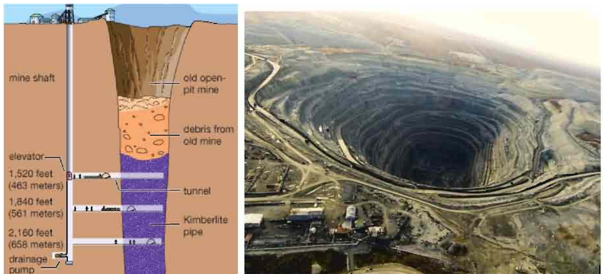
Figure 117. Diamond pipe mining (left) and a diamond mine in Angola
