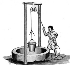
(c) Raising water from a well
