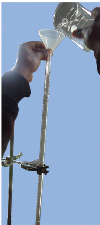
Fig 1.4: Correct filling of burette
