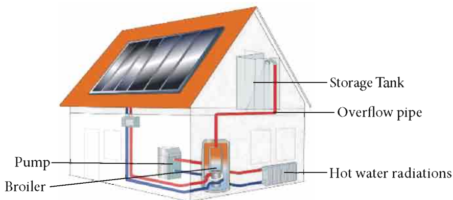
Fig. 3.1 Hot water system in a house
